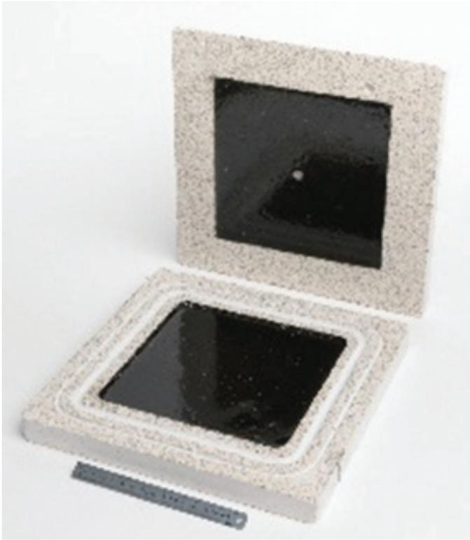
of composites. It can also take liquid samples where the dielectric measurements can be made throughout its cure cycle. Currently there is no such system available commercially.
