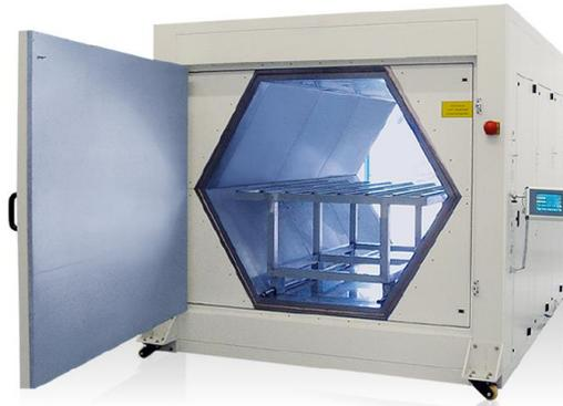
*Fig. 1. Hexagonal-shaped Hephaïstos© VHM 100/100 microwave oven*
