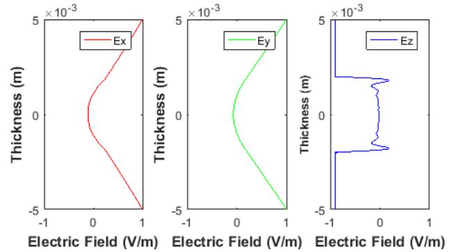
Fig.3. Electric field through the thickness along ( $x_{middle}, y_{middle}, z$ )
