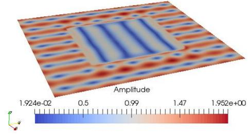
Fig.2. Electric field amplitude in the cross-section ( $x, y, z_{middle}$ )
